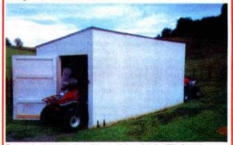
Taylor designed this ``drive-through" storage shed especially for ATV's. It lets him store two 4-wheelers in single file fashion. The 8 by 16-ft. shed has a 4-ft. wide door on each end, allowing him to drive in one end and out the other. ``There's no need to back up or turn around. Makes it easy for my 11-year-old son to get in and out," he says .
