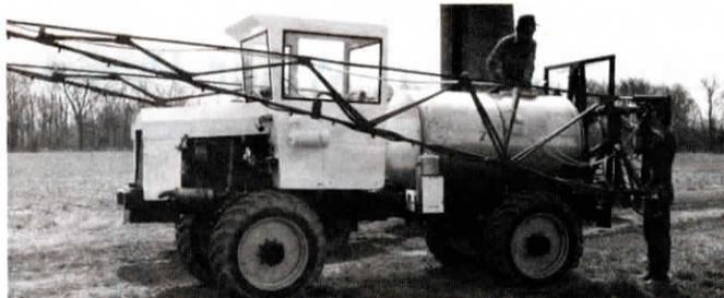
**Sprayer has engine and cab up front, articulated steering, air-bag suspension, and 55-ft. boom.**
