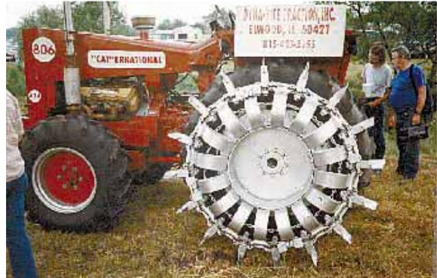
Fold-out cleats are 10 in. wide and 5 in. high. They mount on 2-WD, 4-WD, or front wheel assist tractors with 26, 32, 38, or 42-in. dia. wheels.
