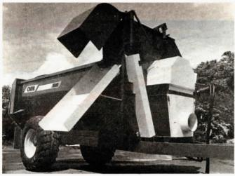
Big up-front rotor feeds manure out through deflector which can be adjusted downward to feed into bunks or upward to spread manure in the field.
