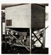
Straw compressing machine makes about 500 lbs. of briquettes per hour using high pressure but no binding material.
