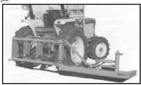
Unlike 3-pt. mounted tree shears, you can drive forward with this sidemounted tree shearer, cutting off trees up to 10 in. in dia.
