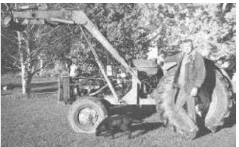
Ellis installed an automatic transmission in his high-speed chore tractor to eliminate the need for a clutch. The result isn't pretty but it gets the job done, he notes.
