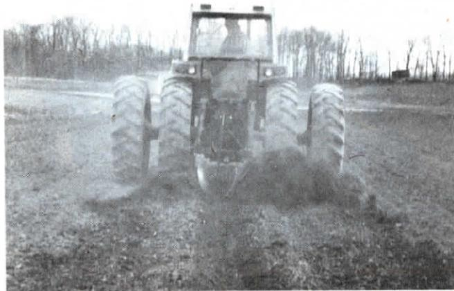
The 3-pt. mounted ditcher uses 2 angled concave discs to dig surface drainage ditches.
