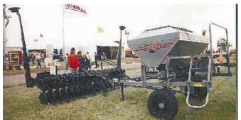
The 4800 air drill is designed to be used with Hiniker's air delivery seed hopper and metering system which mount behind the air drill.
