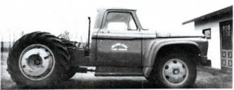
Here's a picture of my "trucktor" built out of a 1966 Ford F-600 with a WC Allis tractor rear end. With the WC rear end, only one transmission is needed to get tractor speeds. I've added a 3/4-ton pickup transfer case to slow the reverse speed down when blowing snow.
