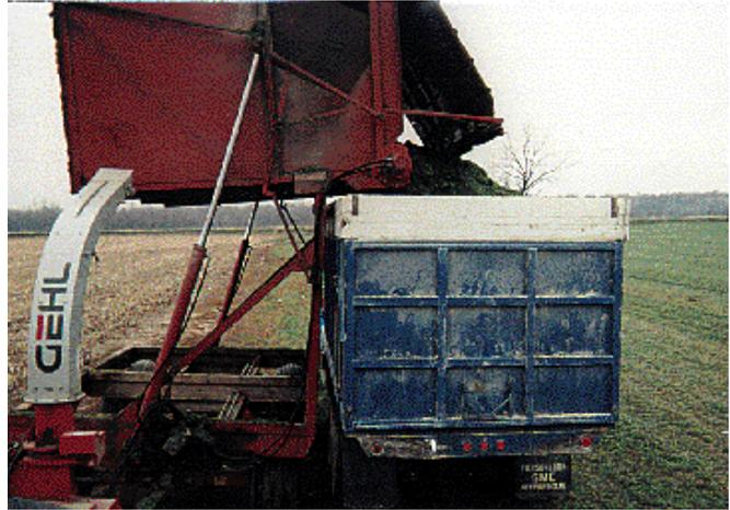
Cover of wagon opens automatically when wagon lifts for dumping. Hydraulic-driven apron chain on side of wagon helps dump into trucks.
