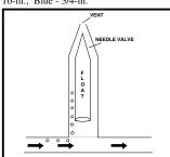
John C. Blundell, Papakura, Auckland, New Zealand: "Here's an automatic air bleed valve I designed to prevent air lock in long water pipes. A short length of pipe runs straight up from the main pipe. There's a vent hole in the top of the pipe which is closed by a float when the main water pipe is full of water. If an air bubble comes along, the float drops, allowing the air to escape."
