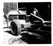
I made a crosscut saw rig out of parts from a Gehl hay crimper, including the gearbox, V-belts, pulleys, power shaft, wheels, and even the tongue - in fact, virtually all the parts are Gehl except for the saw and arbor. The blade is 32 in. dia. Logs are placed on a tipping table. Any tractor with 25 pto hp. or more can power it. Being on wheels, it's easy to trasport and store.
