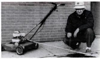
Here's a good way to get rid of moles and gophers. Just remove the muffler from a lawn mower, screw a steel pipe elbow into the engine, and attach a length of electrical conduit to the elbow. Then slip the pipe down into the tunnel and start the engine. To create more smoke in the exhaust, add a bit of diesel fuel to the gas tank.
