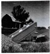
My great grandson came over one day and was playing with sand and a small dump truck. He was putting sand into the truck with his hands. That's when I got the idea of making a toy conveyor. It's made out of wood with a rubber V-belt fitted with plastic cups. You crank the handle to turn the conveyor belt. Children will play with it for hours. I have plans to build it. (John Harp, Rt. 1, Easton, Ill. 62633 ph 309 562-7457)
