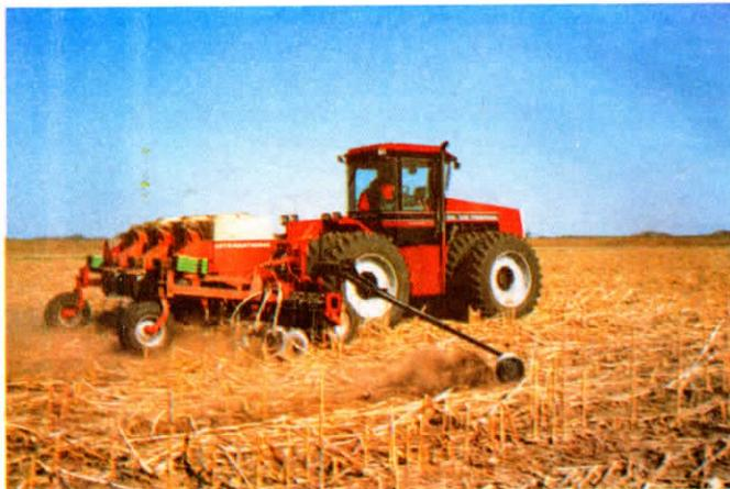
Demmer clamped 24 new Yetter no-till "soybean special" coulters, spaced on 10-in. centers, onto 4-in. sq. steel bar mounted behind toolbar.
