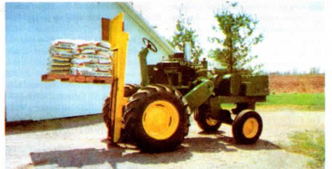
Baldwin cut combine apart and built new frame out of 6-in. channel iron. He bought forklift mast from salvage yard.
