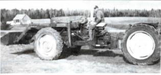
can drive the big front wheels into a snow bank and back out again with no problem," says Murray. "I lengthened the loader 2 ft. It can reach 14 ft, high so I can really pile snow high. I also use it to haul firewood."
