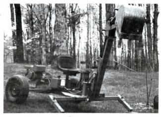
and even lifting shingles up onto a roof. To transport, he moves the wheels from the back of the backhoe to the front and uses a tow hitch at rear. Takes just minutes to switch the wheels - he uses the boom to raise up each side of the backhoe. slip out the wheel and 2 by 4 axle (they come out in one piece) and slip them into axle holes at the base of the boom on the front of the backhoe.
