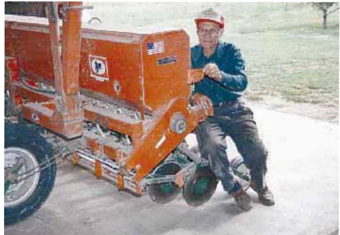
Marker flags attached to the end of drive shaft let Beckmeyer tell at a glance whether drill is still working.
