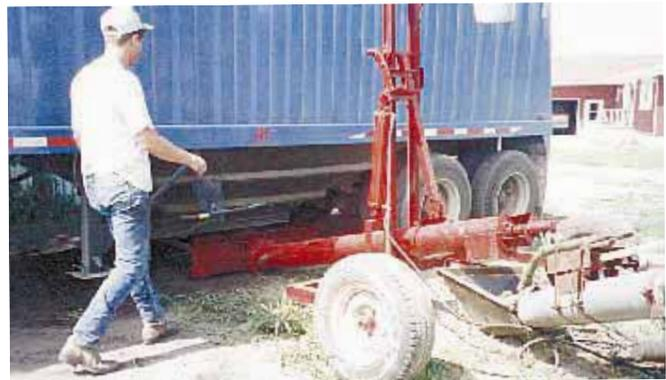
"Shuttle auger" is designed to hydraulically roll hopper down and under grain trailer hopper.
