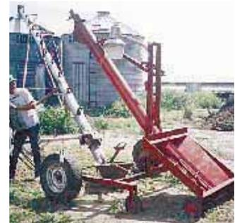
Auger raises up for transport. Note light for night work.
