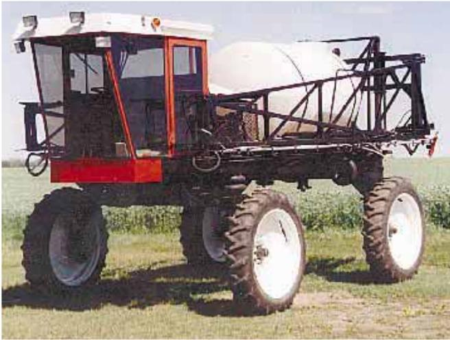
The Frieds' sprayer is powered by a 400 cu. in. short block V-8 engine that's been souped up to 220 hp.
