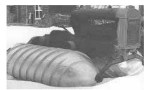
A pair of large flighted pontoons pulled this modified Fordson through snow.
