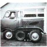
I've built many tractors, 3-wheelers, garden tractors and other equipment over the years. I'm sending along photos of two of my most unusual projects, a 1952 Ford car fitted with half tracks and a "shorty" truck also fitted with tracks. I got the idea for putting tracks on the car when the fenders around the rear wheels rusted out. I cut away the rust and installed a spring-loaded axle with idler wheels that can be adjusted to tighten the
