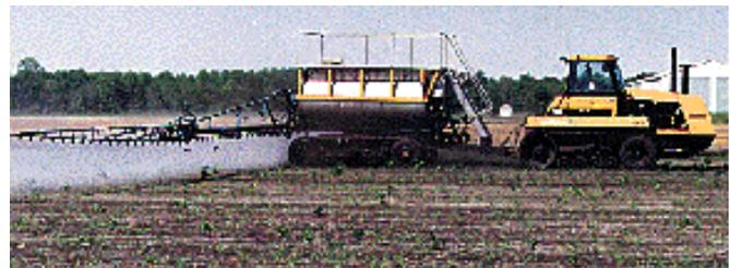
The 14-ft. long, 9-ft. wide tank mounts on top of Caterpillar's 116 Mobile Trac System. When loaded, it weighs about 18 tons but exerts only about 8 psi on the ground.
