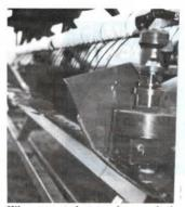
When operated at regular speed, the double stroke sickle drive has twice the cutting action of a conventional sickle. in. on each stroke, allowing for faster cutting speeds and longer section life.
