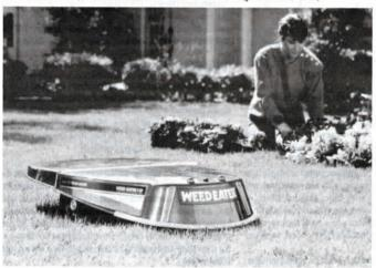
Solar-powered robot mower works its way slowly around lawn, bouncing back from obstacles and moving on to other uncut grass.
