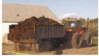
The Kudrnas' spreader is built out of a 40-ft. semi trailer frame and tandem axles.
