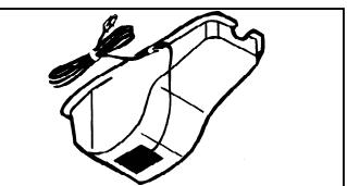
Preheater pad adheres to bottom of oil pan. Can be used on any pan or even on oil barrels.
