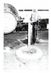
I made a portable grinder by bolting a grinder and electric motor onto the top of a 2 1/2-ft. high pipe. The bottom of the pipe is welded to the rim of a car tire. (Gary Vorce, 32350 Co. Rd., Akron, Colo. 80720 ph 303 345-6703)
