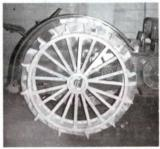
We had trouble driving our steel-wheeled Deere 1929 D in parades or on the road but solved the problem by bolting wood blocks to the wheels between the inside lugs. We bolted them to the rims with 6-in. long 3/8-in. bolts. We pulled the head of the bolts down
