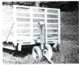
The second photo shows a small utility wagon I built for the farm that uses the front end of a John Deere "B" tractor. The tongue attaches directly to the front-end axle, which casters for easy turning. (Tom Kutruff, Rt. 1, Box 37, Altoona, Penn. 16601 ph 814 944-9205)
