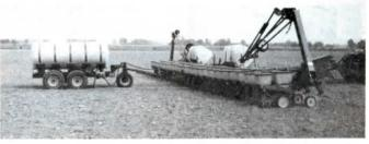
We build sprayer caddies that pull behind planters or field cultivators (Vol. 16, No. 2) and thought your readers would like to see the 1,600-gal. tandem walking beam axle model that we recently built for Merlin Martin, Clayton, Ind. He pulls it behind his 24-row planter and uses it to apply liquid fertilizer. He can plant about 100 acres before he has to stop and refili.
