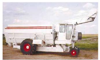
Feed mixer has a 16-ft. long, 6-ft. high box and a 23-in. wide front loader conveyor.
