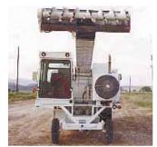
Conveyor auger reaches up to 12 ft. high for silage pits. Moon used a length of 6-in. dia. steel pipe equipped with 5 1/2-in. flighting to build the auger.
