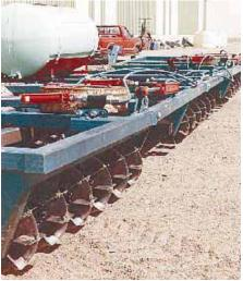
wide knives on 18 1/2-in. The 32-ft. unit is equipped with two rows of cutting wheels dia. cutting wheels. The cutting wheels mount on axles that Fuesz built by mounting pairs of 3 1/2-in. wide steel knives on 18 1/2-in. dia. cutting wheels.
