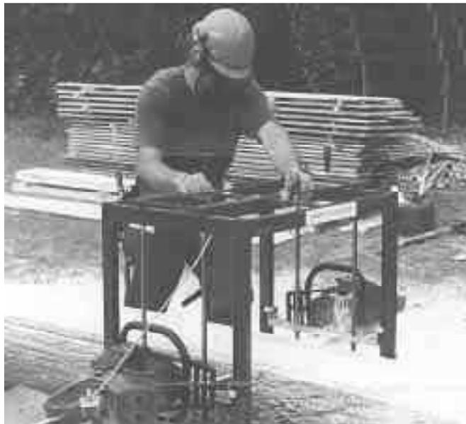
Sawmill's 22-in. wide carriage is equipped with a single chain saw-type cutterbar powered by a chainsaw power unit mounted on either end.
