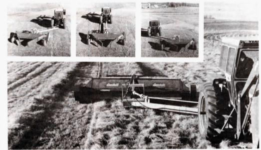
A flick of the hydraulic control lever moves the new Lundell "Swing Tongue" from one side to the other. Eliminates driving over windrows.
