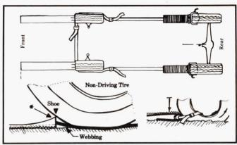
Upper drawing shows arrangement of Strips for vehicle with rear-wheel drive. With straps laid out in this fashion, driver puts transmission in low gear forward, accelerates slowly. After moving car only about 4 or 5 ft., upfront anchoring mats, having maintained their positions on the ground, will lay free and clear behind front
