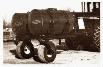
Bumper Jim carriage is available with single wheels (as shown) or with two sets of duals on each side. Up-front unit swivels to follow ground contour.
