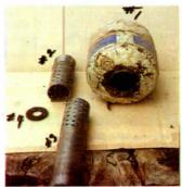
Peters uses hole saw to cut out hole on each end of tank (1). Then he drills 5/16in. holes in pipe to be inserted through tank, and cuts the pipe in half (2 & 3). He welds a thick steel washer between the two pieces of pipe to act as a baffle to diffuse sound out the holes in the pipe (4).
