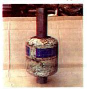
Photo shows pipe inserted into tank, ready to fit over existing exhaust pipe.
