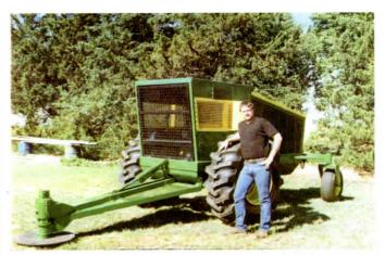
Queal's self-propelled "tree machine" has 30-in. dia. steel cutting blade mounted on -ft. long hydraulically-operated boom.
