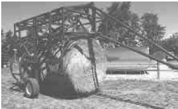
**The 2-wheeled bale mover is equipped with two sets of loading jaws.**
