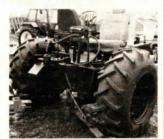
the chassis side rails and are sprocketdriven directly off the driveshaft. They supply power to the backhoe, which is controlled by hydraulic motors that drive chains and sprockets.
