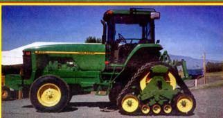
Track system is equipped with idler wheels and rollers that oscillate independently on a 5-point pivot design for better traction and a smoother ride.
