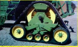
The 1 1/4-in. thick tracks fit rear wheels on any 2-WD tractor.
