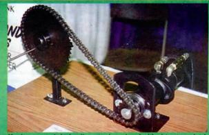
Header reverser's hydraulic motor is equipped with piston-type clutch that eliminates the need for a hydraulic cylinder.
