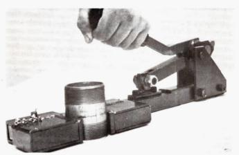
Kwik Klamp works on either plastic or galvanized pipe up to 2 in. in
