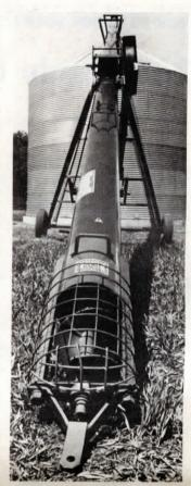
New 8 in. dia. Flexgo augers from Westgo are available factory equipped with rubber at the "input" end.
