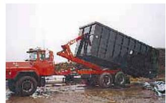
Shuttle arm lets him switch between the tank and a 22-ft. long forage dump box without getting out of the cab.
