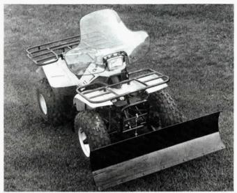
Universal ATV blade plows for moving snow or dirt are available through dealers from Bell Industries. The 48 in. tilt blade, made of 11 ga. steel, has a replaceable wear bar. Mounting bracket can be left on ATV when blade is removed. Blade lifts easily with hand-operated lever.
