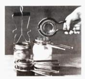
Set includes 2 rubber-lined wrenches, and a Safety Lifter device, shown attached to jar on left.
