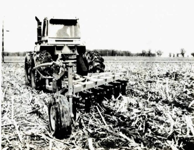
“Paraplow” features legs that slide through the soil at a 45° angle. It leaves the surface undisturbed and residues intact.
