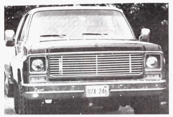
Original grille on this Chevrolet Blazer has been replaced with TOK oil cooler. It's made up of 45 ft. of ½-in. dia. aluminum pipe.
