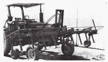
This specially designed mower is used to cut wheat stubble and weeds out from between soybean rows.
