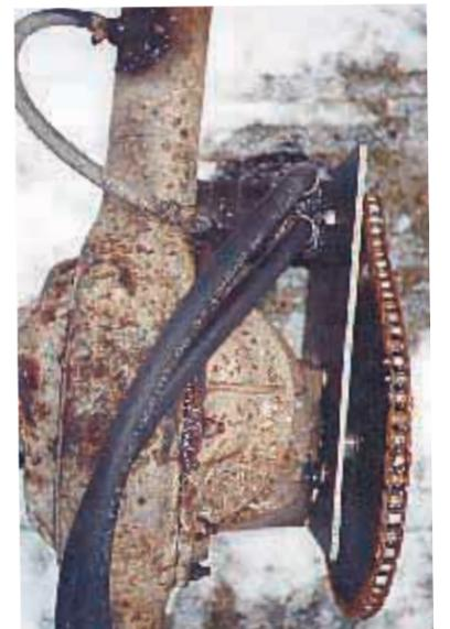
even the coldest weather, he replaced the differential oil with automatic transmission fluid.
