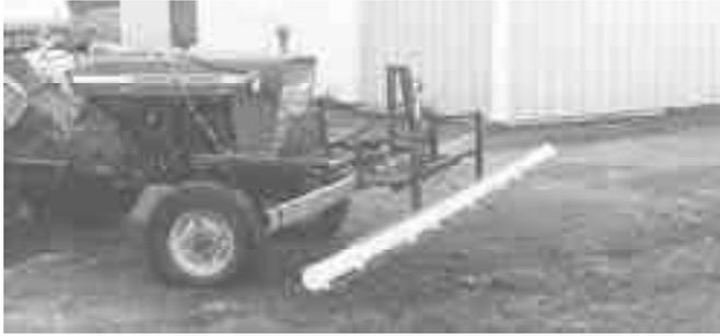
Electrically-charged brass rods mount along a length of pvc pipe. As weeds strike the rods they ground out the electrical circuits and send signals to a control box. It activates spray nozzles mounted on a boom behind the pvc boom.
