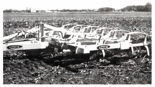
Individual shanks can be tripped manually to raise pairs of shanks, as needed, to lighten the load in tough going, and to match the unit to a smaller tractor.
