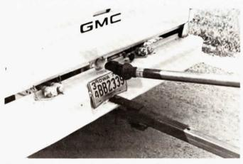
Hydraulic pump mounted under hood has sufficient capacity to power pto and two separate cylinders. Note spools on each side of the pto.
