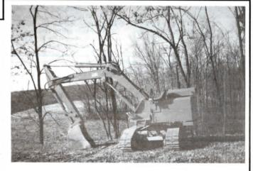
draulic system, made from off-the-shelf parts, is about the only thing that differentiates it from a commercial backhoe. Arnold installed a single hydraulic pump with flow divider on the machine's motor. "That gives it two live oil circuits so I can do all the same operations a commercial unit does," notes Arnold.
