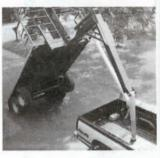
The hydraulic system is powered by a pump driven off the crankshaft pulley on the pickup.
