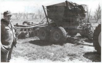
vary the application rate by changing gears on the hopper conveyor chain. The cyclones reduce air pressure created by the fan so fertilizer falls evenly by gravity to the ground.
