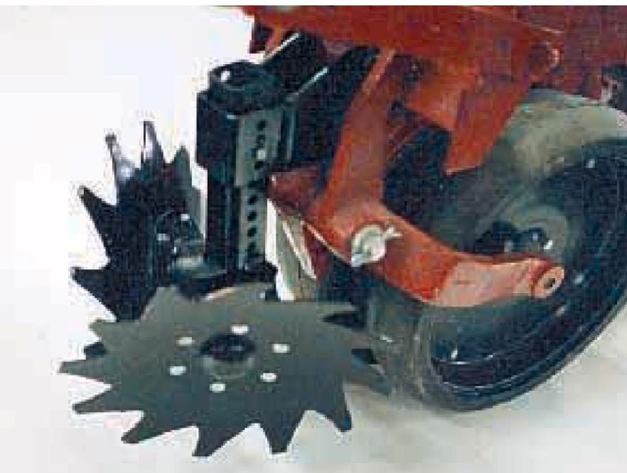
Row cleaning wheels have a concave shape and are equipped with slanted teeth that brush heavy trash out of the way.
