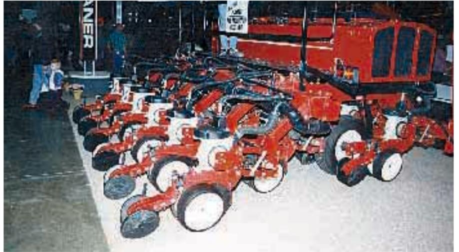
There are three rows of planter units on the new AGCO air planter. Both back rows can be removed to switch from 10-in. spacing to 30-in.
