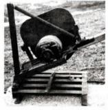
to reduce the size of the 1-in. blade hole. I made a guard to cover the top and sides of the blade out of steel plate.
