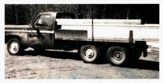
axle has to carry is 3 additional feet of truck bed, and itself. I've carried as much as 5 ton of concrete blocks with no problem," says Beaudoin, noting that he also has a dump box that mounts on the truck bed for hauling gravel or grain. "I've used this truck now for 78,000 miles and I've never had a problem. There's no other pickup in the world that'll match its performance."
