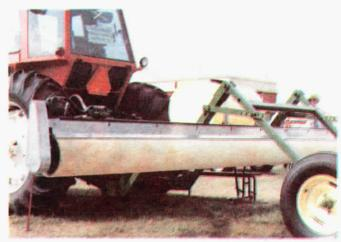
Herbicide is pumped from supply tank mounted on Weed Wiper and fed onto carpet which brushes it onto volunteer corn and other tall growing weeds without touching or spilling on crop below.
