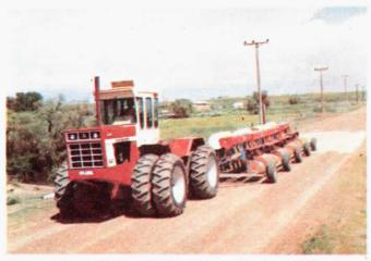
To change from field to road position, just pull a pin and fold swinging section of hitch back to drawbar. Drive forward and drills swing automatically into transport position. No need to unhook tractor or hoses.
